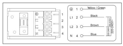
The appliance can be connected directly to the mains by single-phase electrical connection, as shown below.
