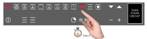
Using the  $\blacktriangledown$   $\blacktriangle$  select "OVEN". At this point, when you select the START key, which is flashing, the program that cleans the inside of the muffle will start.
