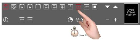
Using the  $\checkmark$  A keys select "STEAM CIRCUIT". At this point, when you select the START key, which is flashing, the program that cleans the inside of the muffle will start.
