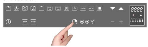
The oven will signal that it is connected to the power mains with a double beep. To set the system time, press the "TIMER FUNCTIONS" button for at least 3 seconds.
