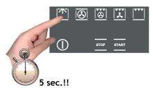
To disable the demonstration mode, touch the light symbol for five seconds: the oven will go to normal operation and be ready for turning on.
