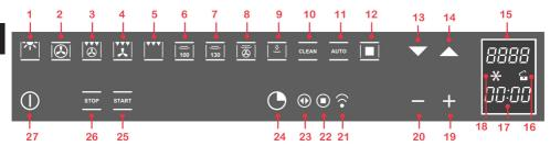
STANDARD COOKING FUNCTIONS: from 1 to 5; SETTING TEMPERATURE, COOKING TIME: 19 and 20;
