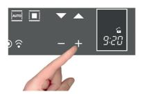
Set the clock with the + and - buttons: during setting the separator dots flash and the time has been set when the dots remain steady on.
