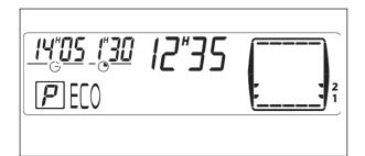
E.g.: 1 hour 30 minutes. When pyrolysis begins, the symbol is displayed in the programmer along with the pyrolysis cycle time.
