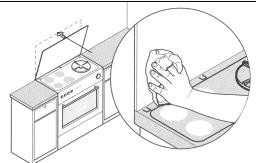
Place the bottom edge of the splashback on the spacers, then push the splashback to the wall and apply firm pressure evenly over the whole surface area.
