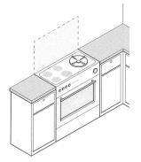
2 Ensure the surface being fixed to is flat, non-porous, dry and dust-free.
