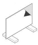
Take the splashback away making sure to keep all corners safe from hard surfaces, then remove the covering from self-adhesive backing. Fit the splashback on top of the spacers.
