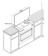
Hold up the back of the splashback to the worktop/wall to check fit. Use the spacers to achieve a good fit.
