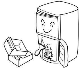
**Caution:** Never use a metal tool or electrical heater for defrosting.
