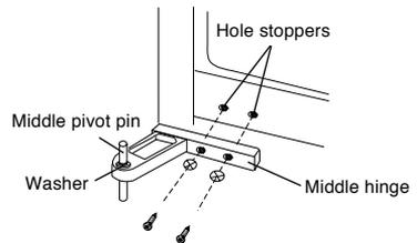
6. Mount the refrigerator door with the top left hole on the down pivot pin of the middle hinge.
