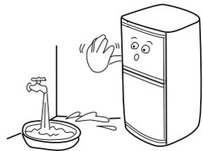
\*Never place the refrigerator in an area with an ambient temperature below zero. Never operate the refrigerator in an open area.
