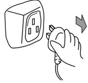
\*Disconnect the power before cleaning the refrigerator.
