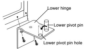
1. Firmly hold the refrigerator door and remove the screws from the right lower hinge. Remove the door and place aside. Remove the lower pivot pin and install it in the left lower hinge hole.
