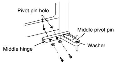
2. Remove the middle hinge and the washer on the middle connection and then the freezer door. Put the door aside.
